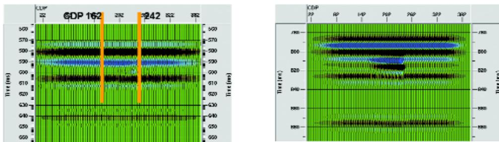
Figure 9. Stacked sections of PP(left) and PS(right) of post-production models with wormholes
