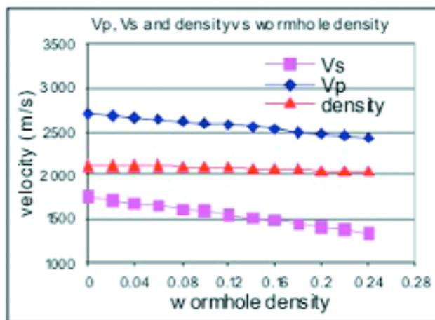
Figure 6. Velocity and density of drainage sands from Murphy's empirical relations vs. wormhole density, where wormhole porosity defined as 50%, reservoir sand porosity as 30%.
