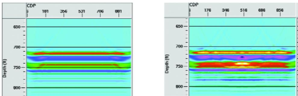
Figure 7. Migrated sections of pre- (left) and post-production (right) models with foamy oil effects.
