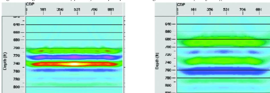
Figure 8 Migrated sections of post-production model using 100Hz (left) and 50Hz (right).
