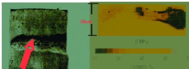
Figure 1. Wormholes simulated in reservoir lab (Tremblay et al., 1999).
