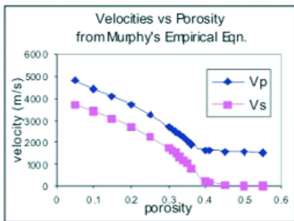
Figure 5. Velocity vs porosity of porous sands
