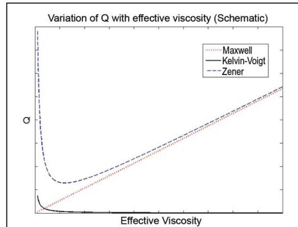
Figure 1. Variation of Q with viscosity for different models from Vasheghani and Lines (2009). The Zener model is the most general and agrees with the lab measurements of Behura et al.(2007).
