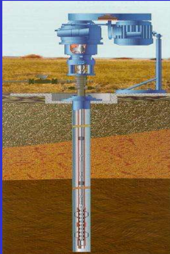
Figure 1 A schematic diagram of a cold production oil pump (courtesy of Kudu Oil Well Pumps)
